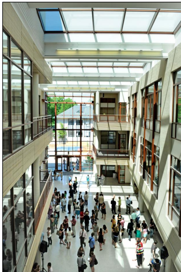
The new School of International Service is designed to achieve LEED Gold. The atrium provides natural light throughout the building, reducing the need for artificial lighting.
